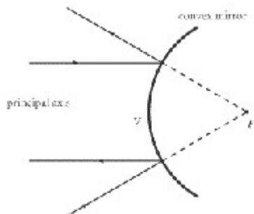
The focal point of a convex mirror is behind the mirror, so light parallel to the principal axis is reflected away from the focal point. Similarly, light moving toward the focal point is reflected parallel to the principal axis. The result is a virtual, upright image, between the mirror and the focal point.
