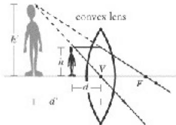
Now the image is virtual and behind the boy on the same side of the lens, meaning that  $d'$  is negative. Consequently, the image appears upright, so  $h'$  and  $m$  are positive.
