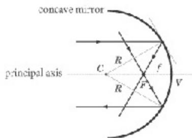
The diagram above shows a “ray tracing” image of a concave mirror, showing how a sample ray of light bounces off it. Though we will take this image as an example, the same principles and vocabulary apply to convex mirrors and to lenses as well.
