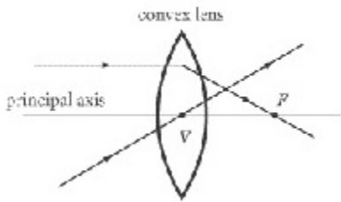
Convex lenses differ from concave mirrors in that their focal point lies on the opposite side of the lens from the object. However, for a lens, this means that  $f > 0$ , so the two equations discussed earlier apply to both mirrors and lenses. Note also that a ray of light that passes through the vertex of a lens passes straight through without being refracted at an angle.
