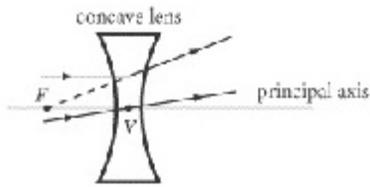
A **concave lens** is designed to divert light away from the focal point, as in the diagram. For this reason, it is often called a “diverging” lens. As with the convex lens, light passing through the vertex does not bend. Note that since the focal point  $F$  is on the same side of the lens as the object, we say the focal length  $f$  is negative.
