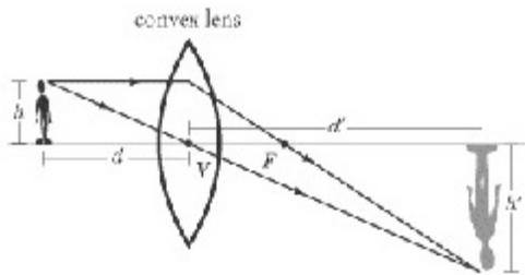
In this diagram, the boy is standing far enough from the lens that  $d > f$ . As we can see, the image is real and on the opposite side of the lens, meaning that  $d'$  is positive. Consequently, the image appears upside down, so  $h'$  and  $m$  are negative. If the boy were now to step forward so that  $d < f$ , the image would change dramatically:
