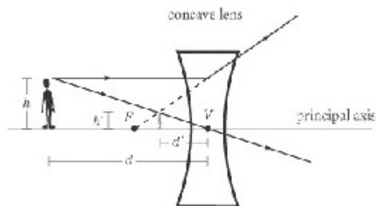
As the diagram shows us, and as the two equations for lenses and mirrors will confirm, the image is virtual, appears on the same side of the lens as the boy does, and stands upright. This means that  $d'$  is negative and that  $h'$  and  $m$  are positive. Note that  $h > h'$ , so  $m < 1$ .
